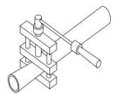
1. Pipe squeezed-off with squeeze-off tool
