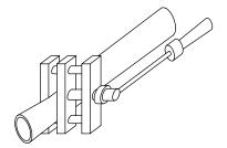
2. Note: After the tool is loosened, you may rotate the squeeze-off tool 90° and reapply pressure to round out the pipe and make installing the support clamp easier. Remove the squeeze-off tool.
